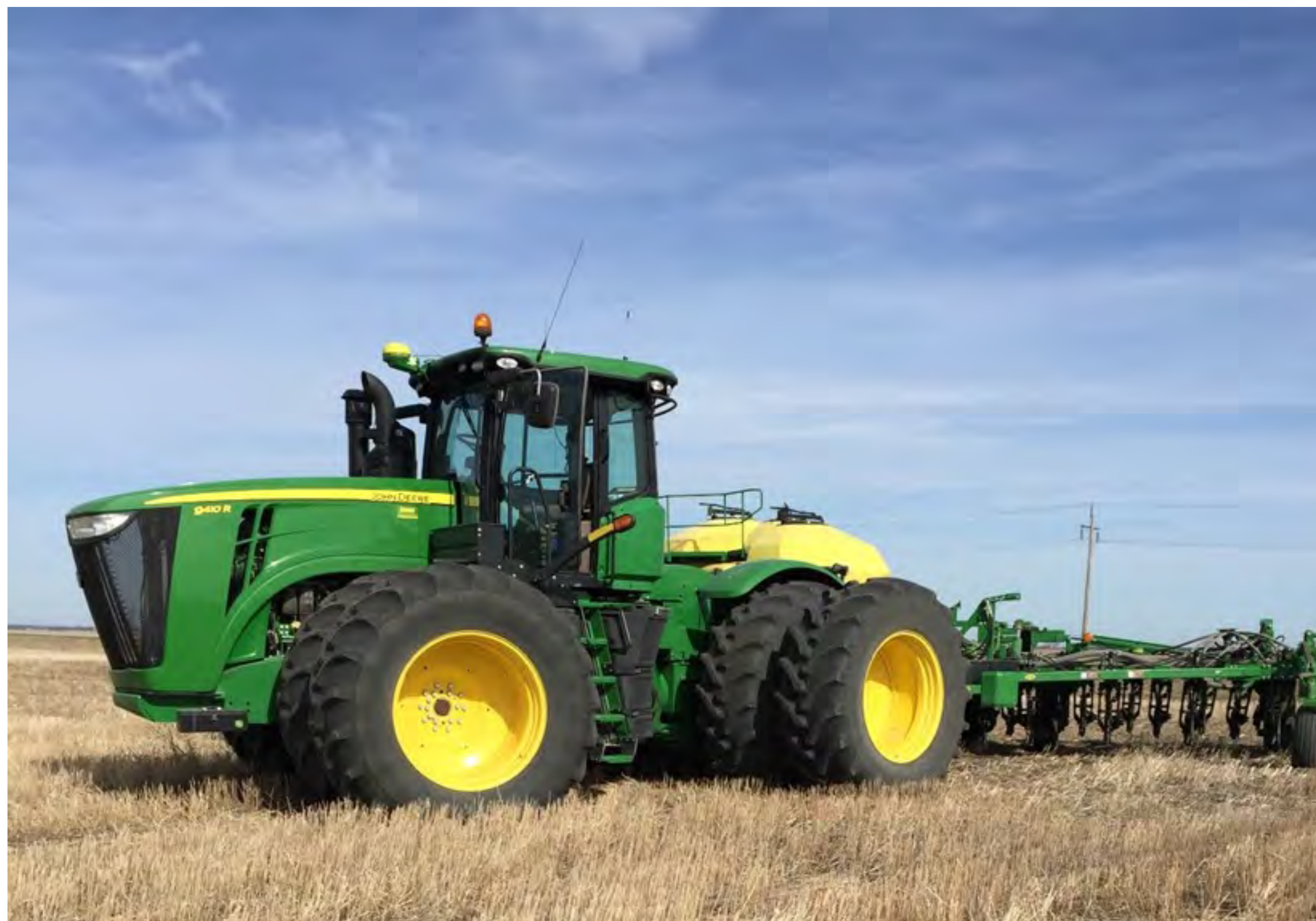
John Deere 9410R with 1910 commodity cart and 1870 air drill with Conserva Pak opener
